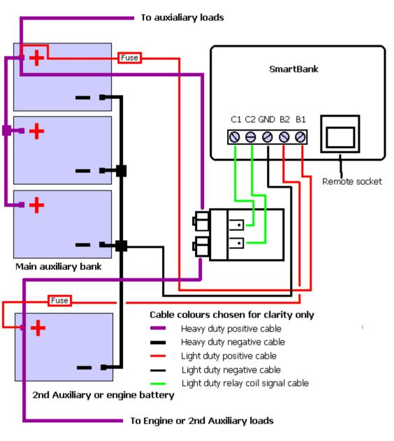
Charge sources and alternators may connect to either Main Auxiliary Bank or to 2nd Auxiliary or engine battery
